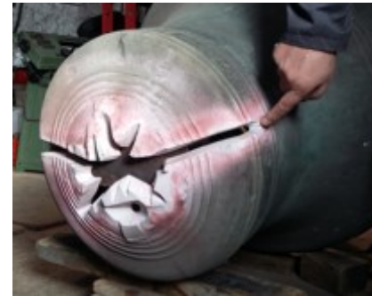
The crack in the fifth bell, ground out and ready for welding
