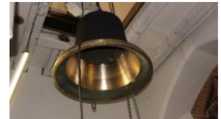
Raising the tenor – tuning work visible on the inside and outside
